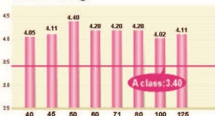
SCOP in Heating
